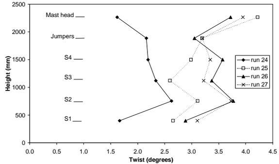
**Figure 17 - Rig twist variation with different rig tunes**
