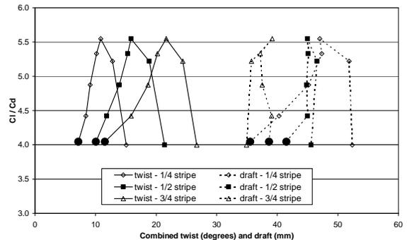
**Figure 16. Variation of  $C_L/C_D$  with twist and draft of combined mainsail and jib stripes at 20° AWA**
