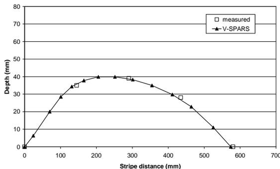
Figure 6. V-SPARS v. known depth of solid mainsail bottom stripe
