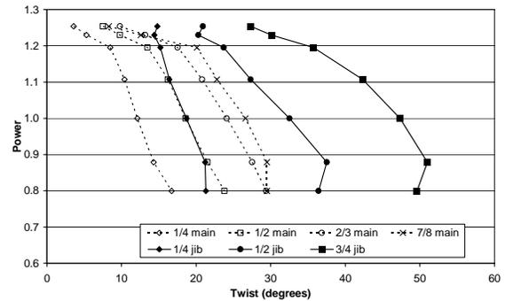
**Figure 15. Variation of *power* with twist of main and jib at 35° AWA**
