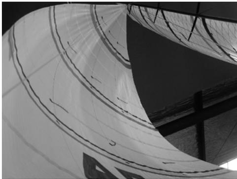
Figure 11. V-SPARS photograph of flying A5 at 60° AWA for stripe validation
