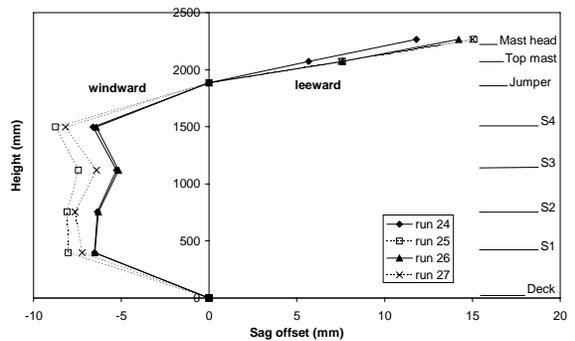
**Figure 18. Sag offset between deck and hounds for different rig tunes**
