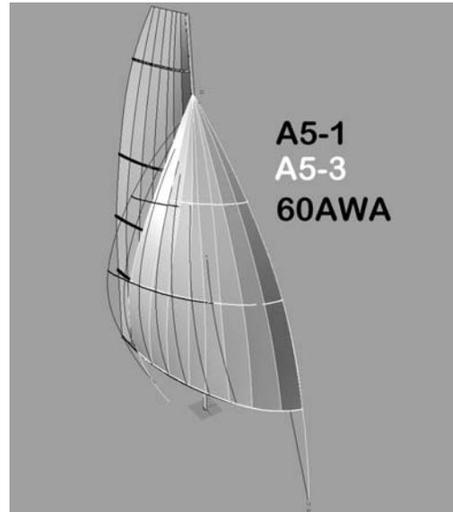
Figure 22. Comparison of downwind flying shapes at 60° AWA
