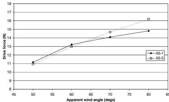
Figure 21. Model scale driving force against apparent wind angle for the A5-1 and A5-3
