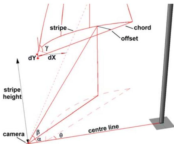
Figure 3. Diagram showing key parameters for stripe shape determination
