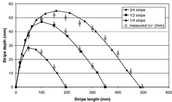
Figure 10. V-SPARS v. known depth of soft jib
