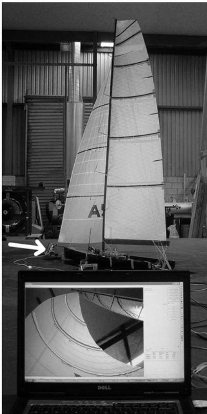
Figure 1. V-SPARS giving real-time downwind flying sail shapes in the wind tunnel (camera location indicated)
