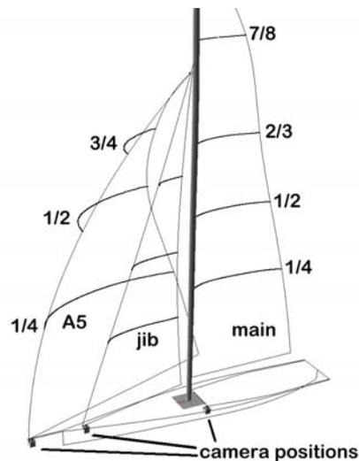
Figure 4. Schematic of camera positions and sails tested
