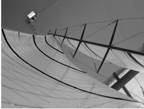
Figure 9. V-SPARS photograph of soft jib for stripe validation
