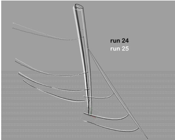
Figure 20. Rig and sail deflection with changing rig tune
