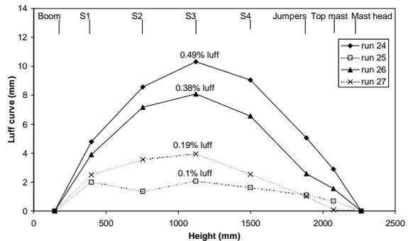
**Figure 19. Luff curve between mast head and boom for different rig tunes**
