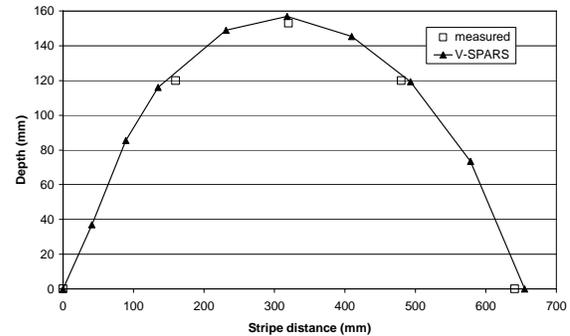
Figure 8. V-SPARS v. known depth of solid spinnaker bottom stripe
