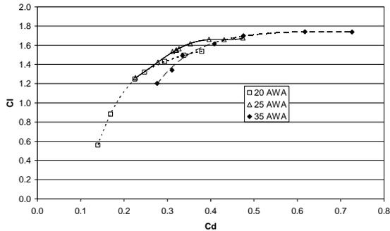
**Figure 13. Lift versus drag coefficient for mainsail and jib combination**
